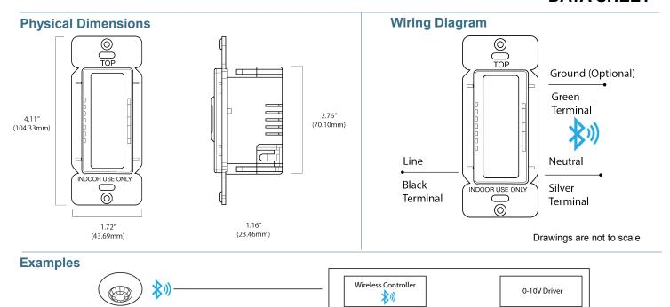
**Bluetooth Luminaire with Integral Sensor**
